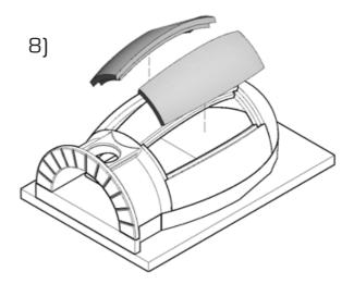
Place the last two shaped pieces into the remaining space so that the locks match.
