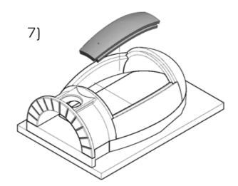
Place the central part of the arch with hole towards the chimney. Shape should be placed on the top of the arch.
