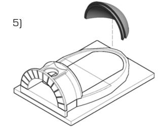
Place the rear arch on the rear plate of the bottom.
