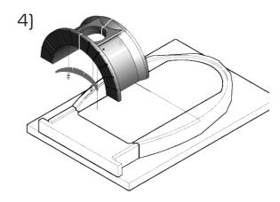
Place the front arch on the front plate of the bottom.
