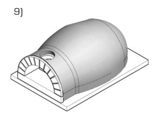
We recommend to isiolate the oven with Ceramic Insulation Biomat and Aluminium foil before enclosing.
