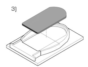
Place the inner plate into the bottom plate cutout.
