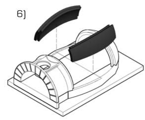
Place the small side arch between the front and rear arch. Side arches should be placed with hole towards the front portal.
